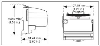
Figure 5. FP-PWM-520 Mechanical Dimensions
